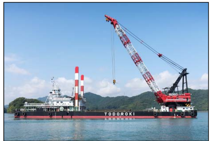
400t吊起重機船
